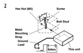
Reinforce the head unit with the metal mounting strap (not supplied). Secure the ground to a wire attached directly to the boat's negative battery terminal.
